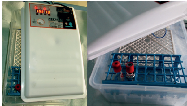
Figure 1. Incubator used to maintain the tubes at a constant temperature of 37°C.
